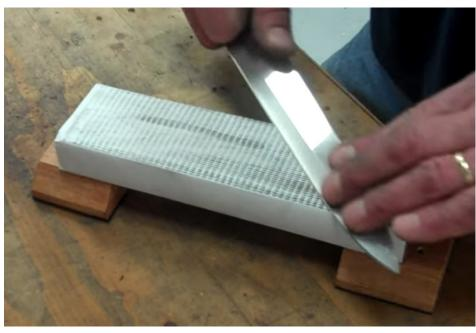
The 'washboard' can be wrapped with sandpaper, abrasive films, or paper which has a compound on it. Or it can be used with plain paper to burnish the steel. Shims hold films / paper against the acrylic surface. It is not much bigger than a bench oil or water stone.
