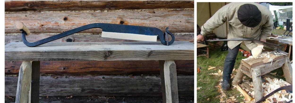
The usual configuration of this large, straight bladed, long handled knife enables you to cut with massive shearing action like a guillotine. The hook at the end is engaged in an eye in a workbench, and allows the user to exert great leverage. The knife back and handle were made of wrought iron to give flexible strength, while the blade had a thin sheet of blister steel laminated on top to give a razor sharp edge. Current versions of this tool are made from high carbon steel.
