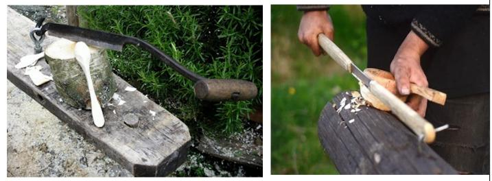
There are also variations in design which change the leverage and range of workpiece height by placing the cutting blade farther from the pivot point and lengthening the overall tool. As you can imagine, this configuration may require extreme physical contortion, fastening the workpiece, enlisting an assistant, or growing longer arms. This seems like a great tool to try out if you can find one at a carving retreat !
