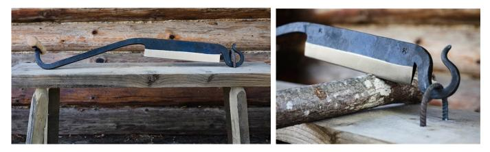
The knife back and handle were made of wrought iron to give flexible strength, while the blade had a thin sheet of blister steel on the top side to give a razor sharp edge.
