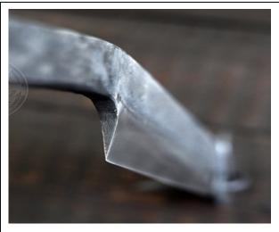
There is limited ability to steer an active cut; and some designs of the tool feature variations to the bevel which yield a greater degree of controlled steering.
